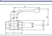
TECHNICAL FEATURES: Temperature limits: for fluids from -20°C to +130°C (peak temperature +150°C) for gas from -20°C to + 60°C
